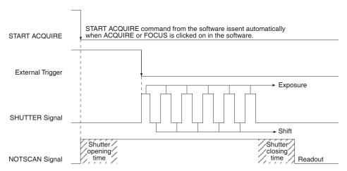
Figure 23. Single Trigger Timing Diagram
